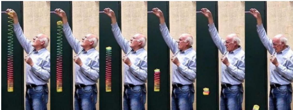
Figure 2: The behaviour of a slinky dropped from being held at the top. Notice the bottom of the slinky does not move until the top has “caught up”.
