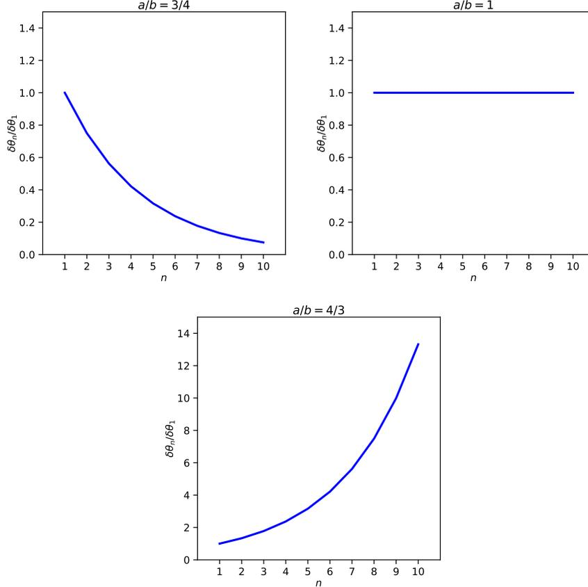
Figure 6: Displacement profiles of the zero-modes for  $a = 0.75$ , and  $b = 1$  (left),  $a = b = 1$  (middle) and  $a = 1$  and  $b = 0.75$  (right).
