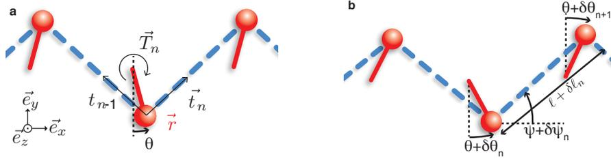
Figure 5: Sketches. (a) torque balance on unit cell  $n$ . (b) Geometry of the system in the deformed configuration.
