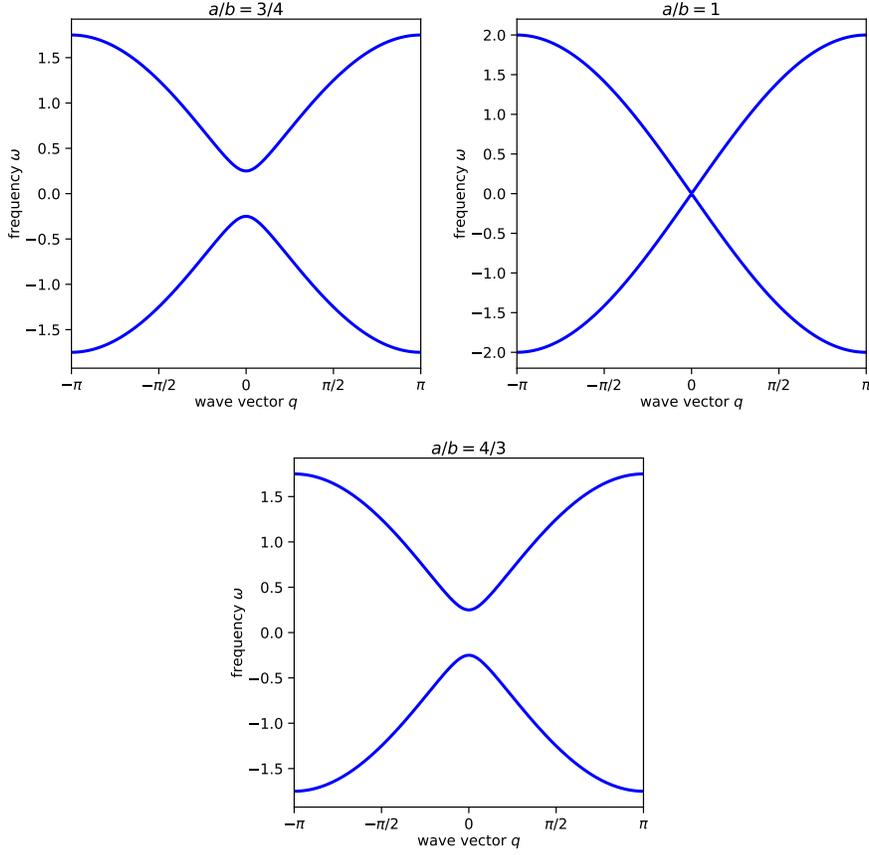
Figure 7: Dispersion relation  $\omega$  vs.  $q$  for  $a = 0.75$ , and  $b = 1$  (left),  $a = b = 1$  (middle) and  $a = 1$  and  $b = 0.75$  (right).
