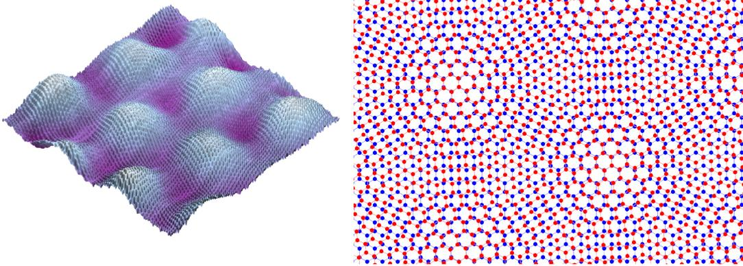
**Figure 3:** (left) Scanning tunneling microscopy (STM) image of twisted graphene. (right) Schematic Moiré pattern created by rotating two graphene layers (red and blue) relative to each other.
