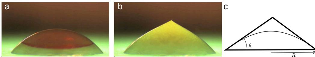
**Figure 9:** (a) Photograph of a partially frozen drop, after it is placed onto a cold surface. The bottom part of the drop has turned into solid ice (green), while the top part is still liquid (red). (b) Photograph of the fully solidified drop, exhibiting a conical tip. (c) The tip formation is modelled by a transformation from a liquid “spherical cap” to a solid “cone”. Both the cap and the cone have the same base radius  $R$  and the same angle  $\theta$ .
